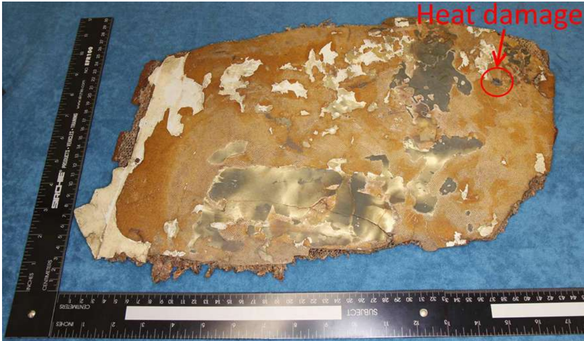
Figure 2: Larger composite panel showing discrete area of heat damage
